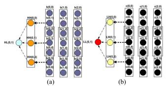
Fig. 6: The detailed operations of the second stage 1-D DWT. (a) The HF (HH and HL) part operations. (b) The LF (LH and LL) part operations.
