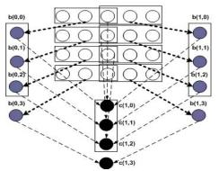
Fig. 5: The detail operations of the first stage 1-D DWT.
