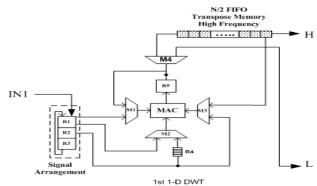
Fig. 7: The architecture of the first stage 1-D DWT.
