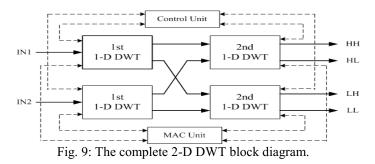
The multilevel DWT computation can be implemented in a similar manner by our proposed high performance 1-level 2-D LDWT. For the multi-level computation, this architecture
